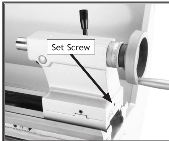
Figure 32. Tailstock off-set adjustments.
