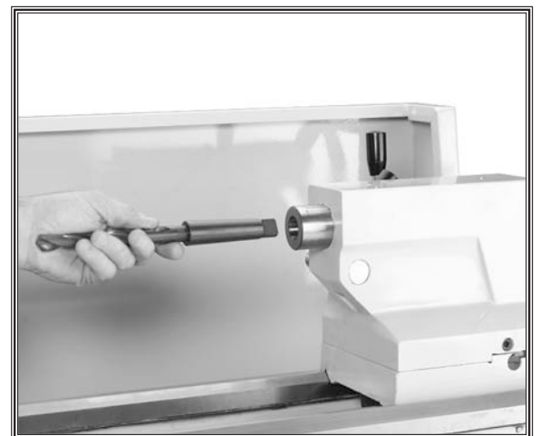
Figure 31. Tapered shank drill fitting into quill taper.
