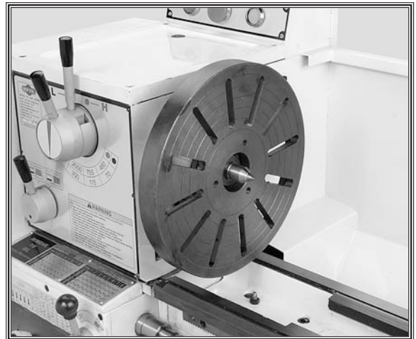
Figure 39. Typical faceplate and dead center setup.
