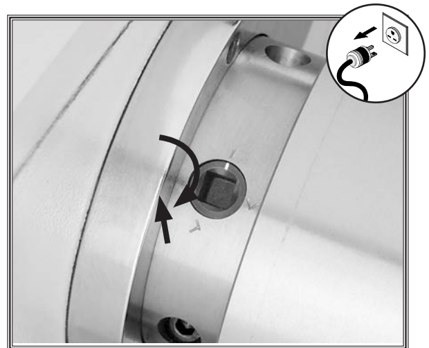
Figure 21. Tightening the cam-locks.
