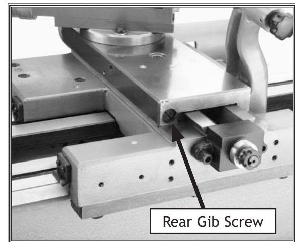
Figure 70. Rear cross feed gib screw.
