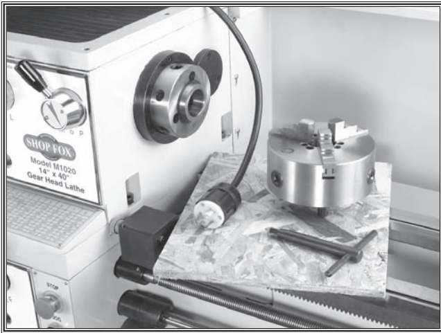
Figure 1. Protecting the bed ways and working safely with electricity.
