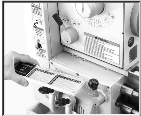
Figure 64. Quick change gearbox cover.
