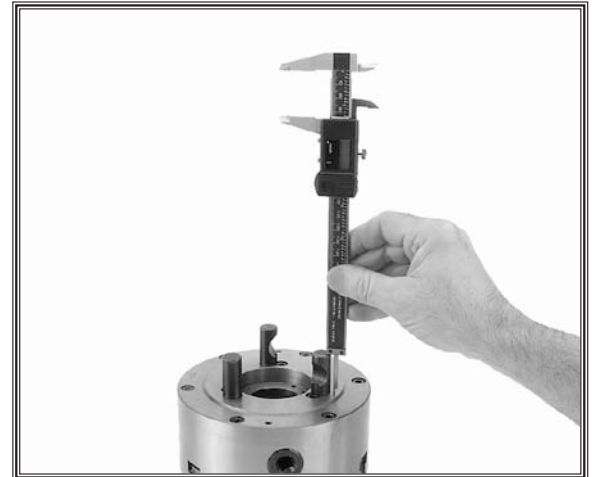
Figure 20. Measuring height of cam-lock studs.
