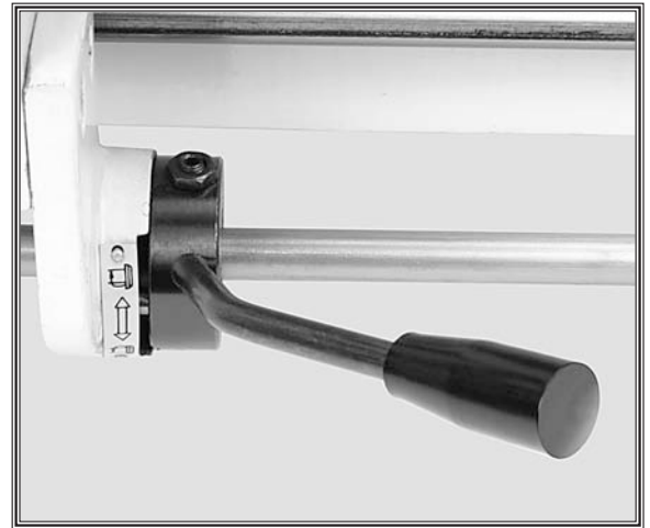
Figure 49. Spindle ON/OFF switch.
