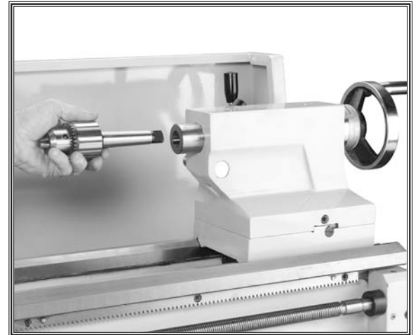
Figure 30. Setting up tailstock for drilling.
