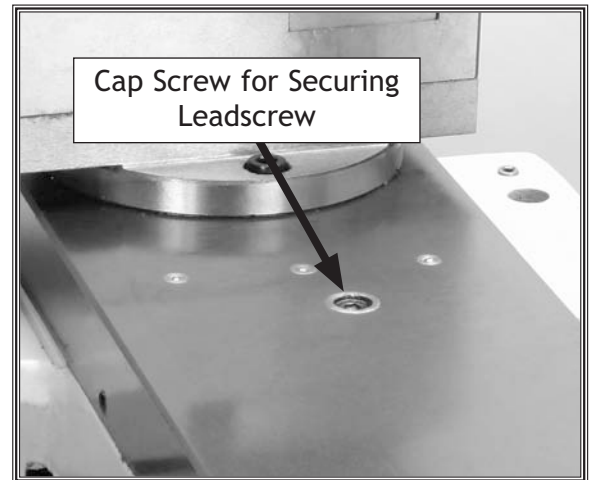
Figure 67. Cap screw for securing the leadscrew.
