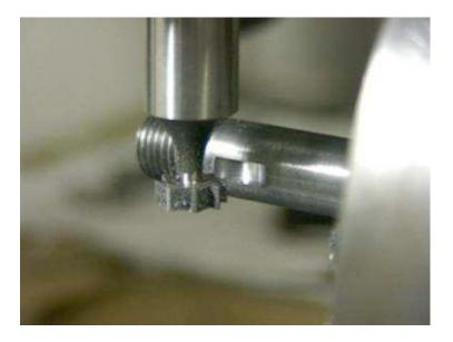
Finally, I used a die to form the 3/8" x 20 tpi threads (ran the die to the appropriate depth, then turned it over and ran it again to cut good threads for the entire length.)
