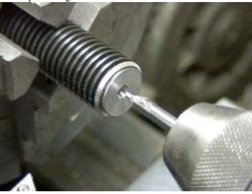
I placed an old feeler gauge between the dial indicator and the rod to center the work in the chuck, then drilled the 60 degree tailstock hole. I loosened the chuck, and mounted the rod on a live center, and re-indicated the other end in the chuck. I used a carbide insert to rough cut, and HSS to finish cut the work.
