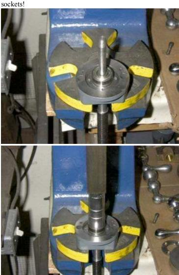
You can, now, screw down the retainer. Attach the whole assembly back into the knee. Actually, before you tighten, you'll want to liberally coat the leadscrew with Vactra 2, and run the nut onto the screw. Screw back and forth the full length of travel to make sure the nut is able to travel fully to both ends.
