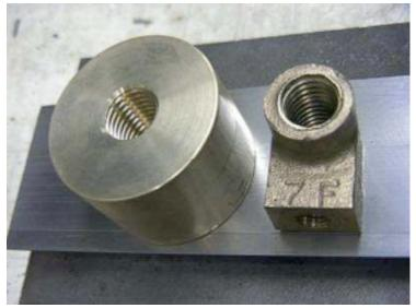
My main concern was whether there would be enough material to mill a sufficient-sized flat to mount the nut without some hokey shimming strategy. The original part 'floats' on a couple of precision washers, which had imprinted themselves in the bottom of the bronze nut over 40 years which made measuring a challenge.
