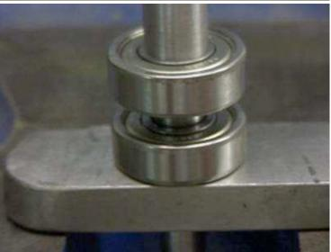
Insert the spring clip into the housing, and press the rod with both bushings into the housing. Thank goodness for ½"
