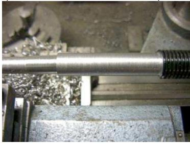
I extended the 'free' (non-machined) end of the leadscrew about 1/2" just because there was room. Also, I left a couple extra threads on the machined end. Basically, the new nut is about 1/4" longer than the old, and I wanted to make sure I engaged all the threads wherever possible. I used a 1/8" keyway cutter for the new woodruff key.
