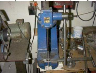
I suppose you could carefully hammer the bearings in place with wood blocks, but I'd be very careful. Start the rod into the first bearing, then carefully seat against the shoulder. Add the thin washer, then start the second bearing and seat against the first.
