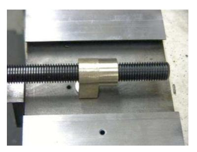
However, I was to learn later that I had one more machining operation before I was finished. Due to the increased diameter of the screw, the 'nose' interfered with the knee when extended furthest away from the column. To rectify this, I relieved some metal off the nut (about .065").
