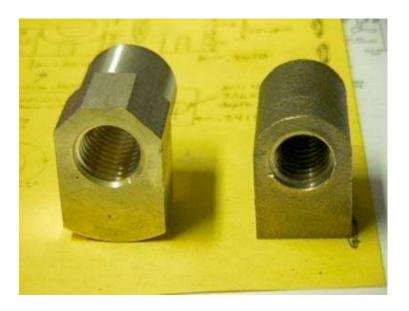
I ground on the nut a little to round things out, then mounted it upside-down in my rotary chuck to begin milling the flat that will mate to the saddle. After completion, I prepared for drilling, then center drilled, then tapped with a 7/16° x 20 · ·
