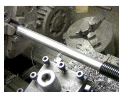
I paid extra attention to the surfaces where I would press-fit the bearings, because they have to be spot-on.
