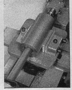
Vise table alone (No. W68-2A) holding long piece for boring in Atlas 10" lathe.
