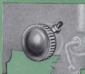
Heavy-duty spring, housed in cap shown at left, controls the tension on feed pinion shaft. Provides any desired tension.
